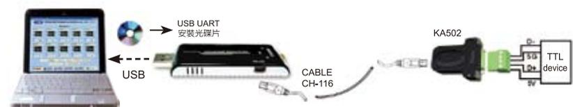
Taking KA301 USB terminal to insert the USB socket of PC and connecting CABLE (CH-116) with KA502 connector, and then connecting the opposite site of KA502 with the TTL device of controller.
