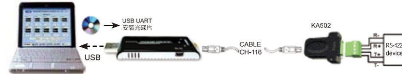
Taking KA301 USB terminal to insert the USB socket of PC and connecting CABLE (CH-116) with KA502 connector, and then connecting the opposite site of KA502 with the RS-422 device of controller.
