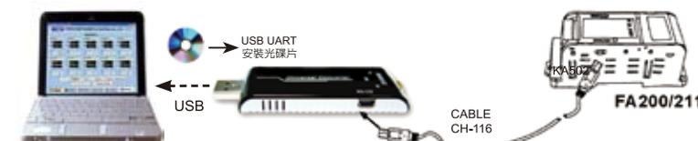
Taking KA301 USB terminal to insert the USB socket of PC, and then connecting CABLE (CH-116) with FA200-211 Temperature controller.
