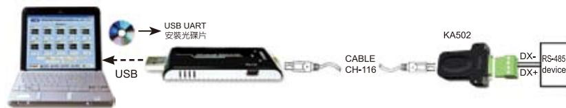
Taking KA301 USB terminal to insert the USB socket of PC and connecting CABLE (CH-116) with KA502 connector, and then connecting the opposite site of KA502 with the RS-485 device of controller.
