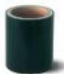
When attached to the surface of an object with unknown emissivity or a glossy object, this tape provides an emissivity of 0.95, enabling accurate non-contact temperature measurement. Emissivity on the PT-2LD can be switched between two levels. Set the emissivity to 0.95 (DARK) for use. The tape is built with material resistant to heat up to 250°C (482°F).
