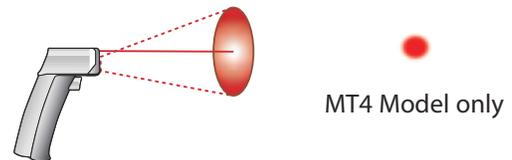
**Laser Point** Single-point laser indicates the approximate center of the target spot.
